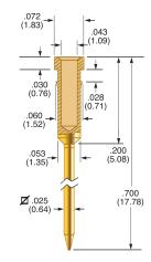
SIP-90-4 Materials: Brass, gold plated Mounting Hole Size: .055 (1.40) Applications: Designed for use in original Factron interface panels. SIP-90-4 replaces SIP-90-1.
