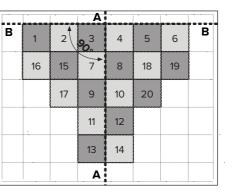
6. Final cuts and completion of the perimeter floor tiles (see clause 3.6) can be done only after you have laid all floor tiles. Ideally, after several hours from the application. When cutting the perimeter floor tiles, allow for a 5 mm gap from any fixed points (e.g. columns, racks and walls). This joint can be pointed with flexible sealant or covered with a strip.
