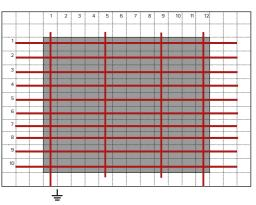
8. After installation, the floor must be properly cleaned (clause to obtain correct values during the conductivity tests. If the current floor has been already earthed, the floor must be insulated.
